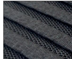
Alternating combination of knitted spacer and net structure on seat covers.
